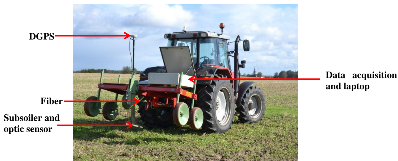
Figure 1. The on-line visible and near infrared (vis-NIR) soil sensor attached to the three point linkage of a tractor [16].
