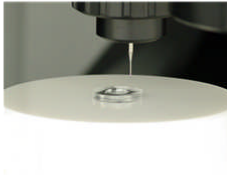
Figure 4. Polymer disc positioned onto the ceramic reference platen of the Zeiss CMM machine. The image shows also the tactile scanning probe.
