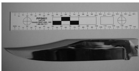
Figure 1. Knife test blade, the UK Home Office number 5 design [17]
