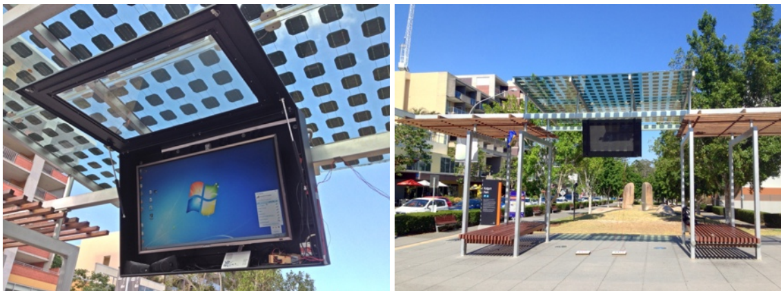
Figure 5.4: The main screen used for testing, deploying and evaluating Vote With Your Feet at a bus stop. Its enclosing case is water proof and also protects the hardware from vandalism.
