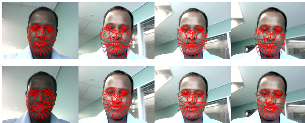
(b) Tracking with sequence for frames 1, 70, 100, 130 of person who is walking along a passage in a building.
