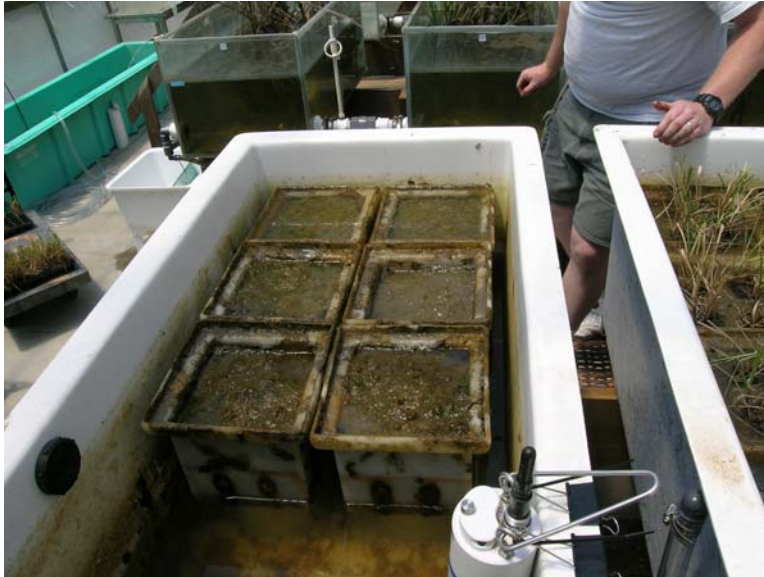
Figure 39: Sediment trays deployed into mesocosms
