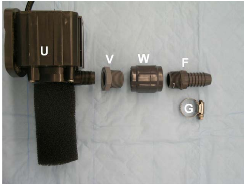
Figure 20: Submersible pump assembly
