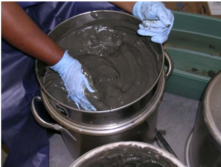
Figure 36: Sediments being sieved (3mm sieve)
