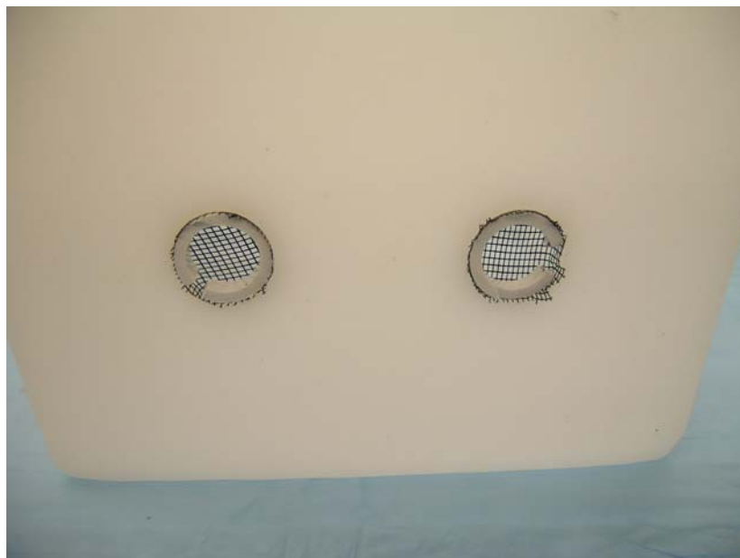
Figure 15: Sub-surface holes with snap rings and mesh -- completed
