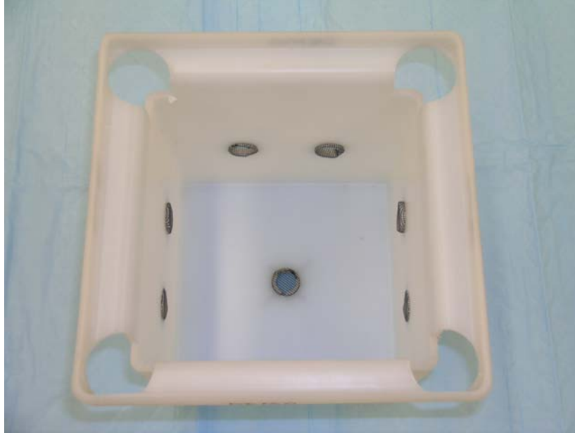
Figure 16: Top view of surface drainage holes
