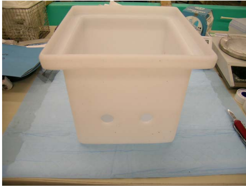
Figure 13: Sediment tray (2 gallon) with drain holes drilled into sides
