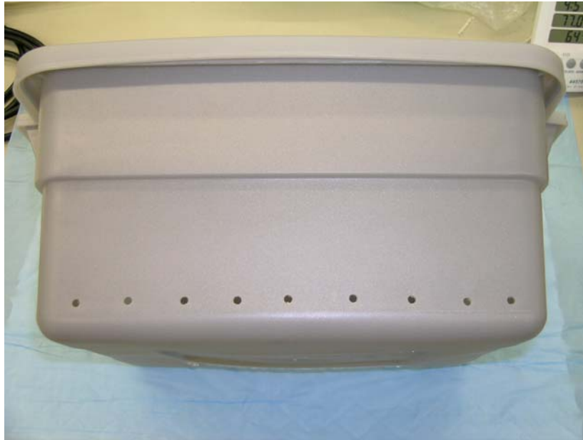
Figure 18: Aeration holes along bottom edge of aeration box.
