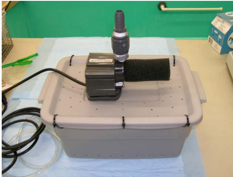
Figure 24: Assembled aeration box/pump support
