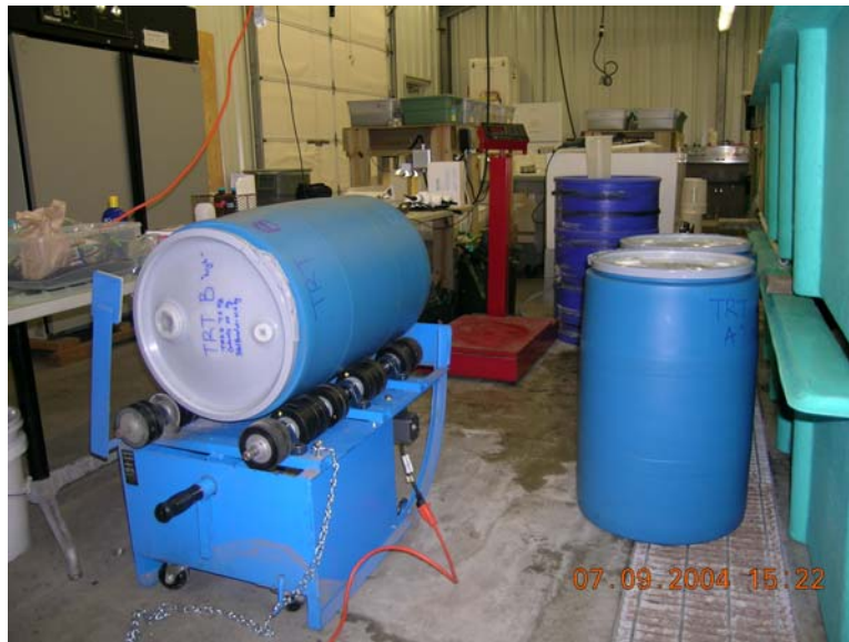
Figure 37: Sediment homogenization on drum rotator
