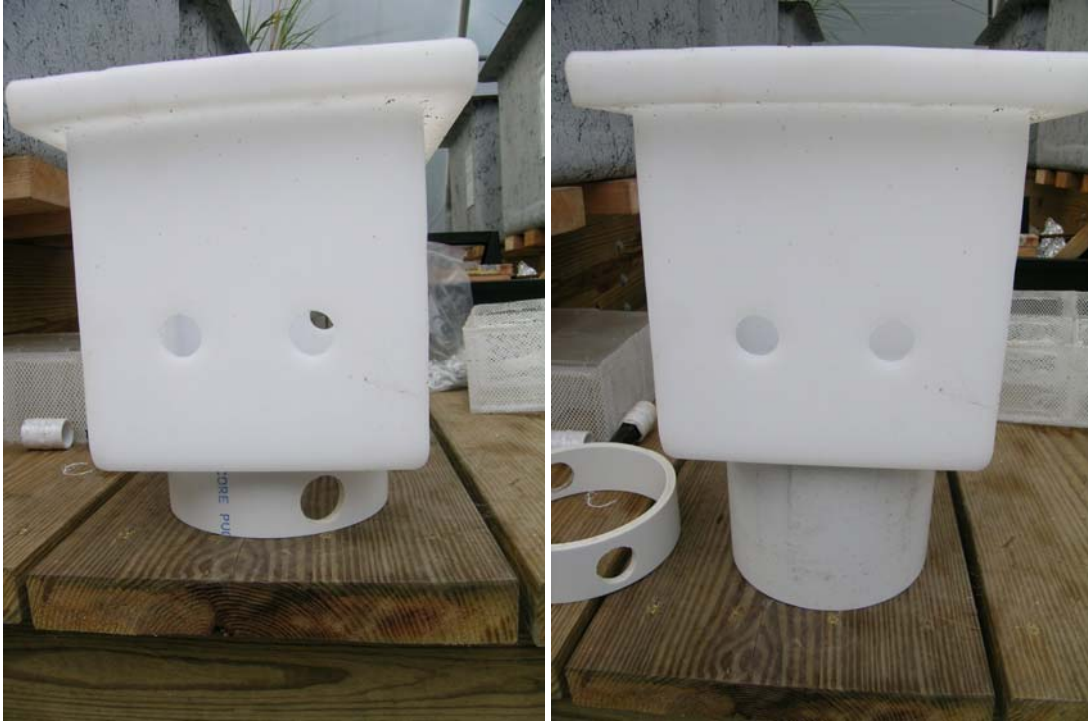
Figure 32: Sediment tray with 2" and 6" high stanchions.
