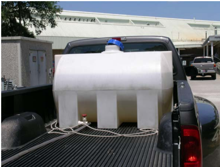
Figure 34: Portable seawater collection tank
