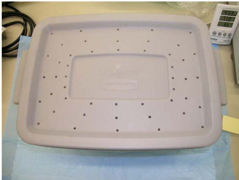
Figure 19: Aeration hole pattern for aeration box lid.
