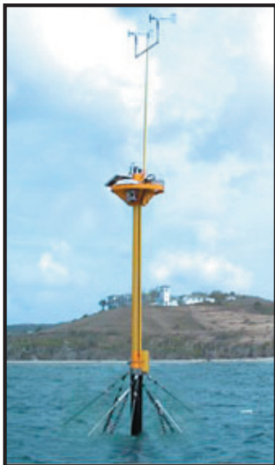
Figure 3.1. NOAA/AOML Coral Reef Early Warning System (CREWS) station.
