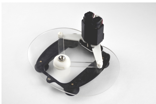
Figure 1: The 2-DoF Haply force-feedback device
