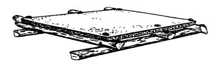
Figure 1. A large "casita" constructed with a frame of thatch palm and roof of cement.
