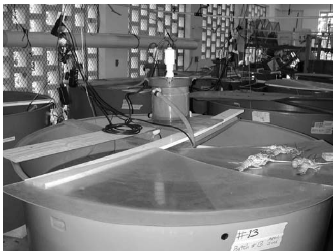
Figure 1. 1500-liter aquarium at the South Florida Regional Laboratory equipped with heaters and an 18 watt ultraviolet sterilizer.
