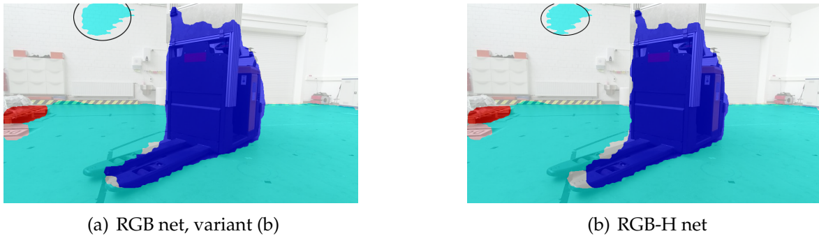
Figure 4.15: A visual comparison of the RGB- (left) and RGB-H (right) net outputs shows that the segmentation results are quite similar. On the right the incorrectly labeled region ("floor" instead of "void") nearby the ceiling is slightly smaller (marked by a black oval).
