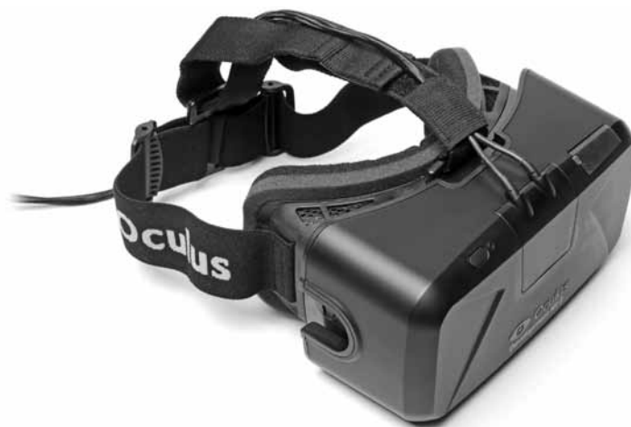
Figure 11, The Oculus Rift DK2, a head-mounted display.
