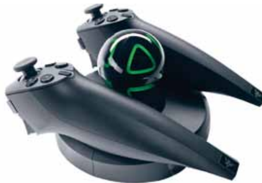
Figure 3 , the Razer Hydra a current game controller, which uses magnetic tracking.
