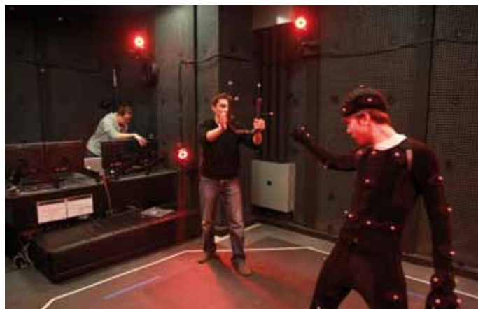
Figure 6, A motion capture studio, showing actors in motion capture suits with passive markers for optical tracking.
