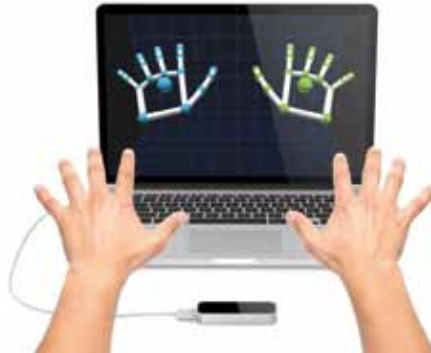
Figure 10, The Leap Motion, a gesture recognition device.
