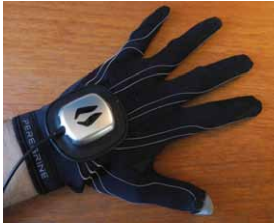
Figure 9, The Peregrine Glove, a touch based data glove.
