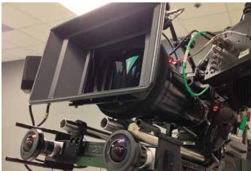
Figure 13, The nCam camera tracking system (bottom) mounted onto a movie camera.
