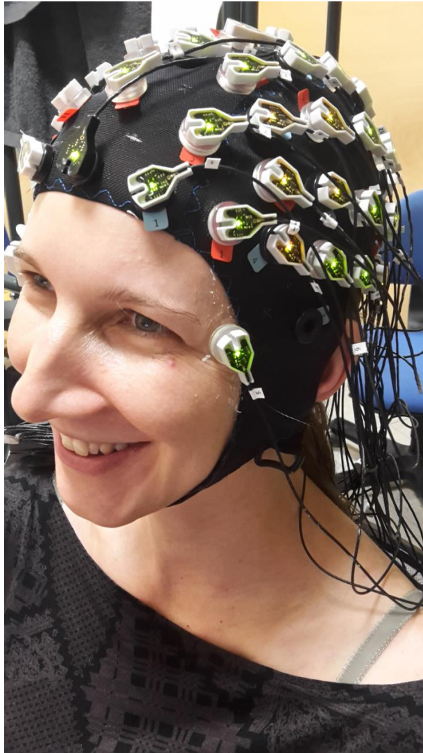
Figure 26. ActiChamp system during installation of a happy subject.
