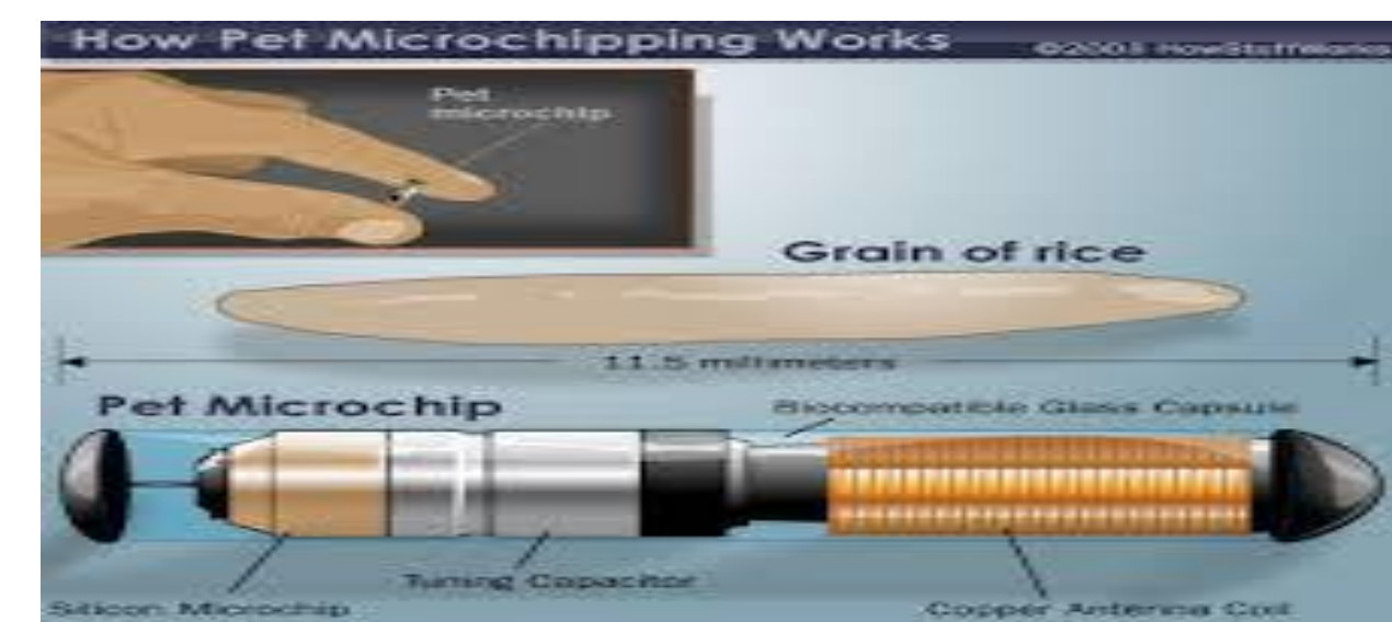
Figure 2 : Diagram RFID microchip (Privacyliving.com)
