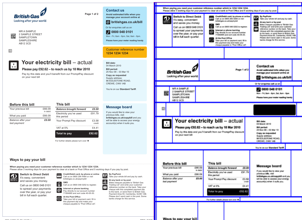
Figure 5.28: HVTO Segmentation: The sample of a bill (British Gas, 2013) (left) and result of horizontal/vertical segmentation (right)
