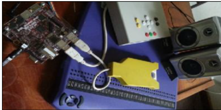
Figure 6.8: Reading system connected to Braille terminal
