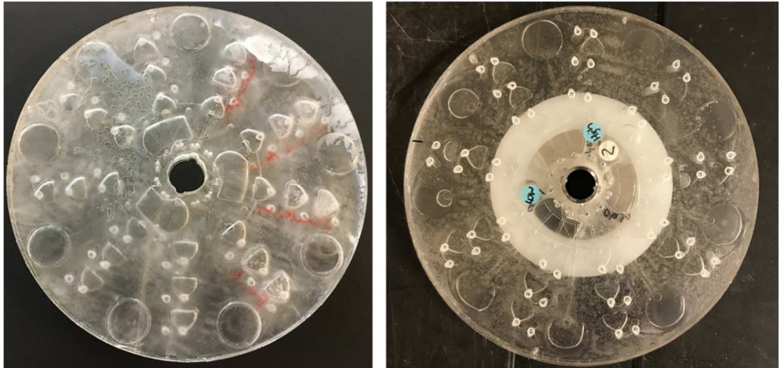
Figure 6.13: Issues associated with the optical transparency of the discs during transportation.
