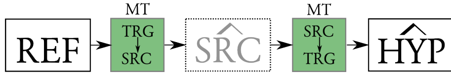
Figure 4.7: The flow of creating synthetic data for APE, proposed by Junczys-Dowmunt et al. (2016). The reference side of a parallel corpus is translated to the source language, using an MT system from \text{TRG} \rightarrow \text{SRC} . This "pseudo-source" is then translated back into the target language using a \text{SRC} \rightarrow \text{TRG} MT system. The resulting "pseudo-hypothesis" should be close to the reference, but is likely to have noise introduced by passing through two MT systems.
