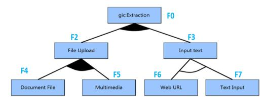
Figure 5.4: Feature Model of gic: Extraction
