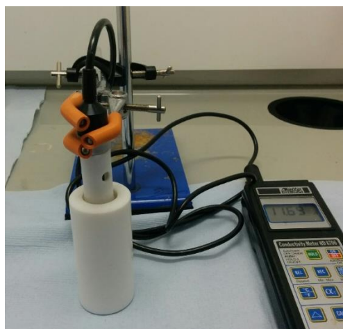
Figure 3.2: HD 8706 Conductivity meter with custom built PTFE probe guard and custom built PTFE sample cup
