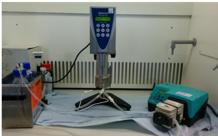
Figure 3.1: Brookfield DV-II+ Pro viscometer with temperature controlled recirculation unit used to maintain solution temperature at 25°C during testing
