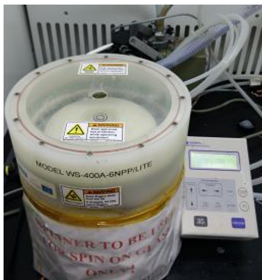
Figure 2.3. WS-400A-6NPP spin coater from Laurell technologies
