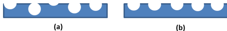
Figure 5.8. (a) actual pore formation on surface (b) pore formation considered for calculation
