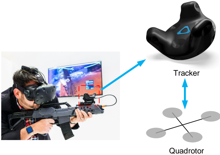
Figure 1.7: An idea to use HTC VIVE trackers to do robot localization
