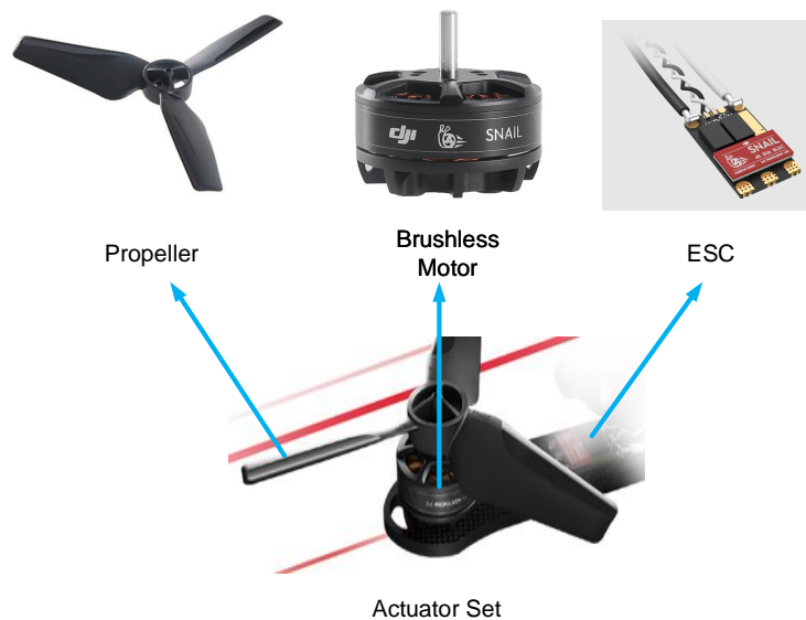
Figure 1.6: Actuator Set (Propulsion System)
