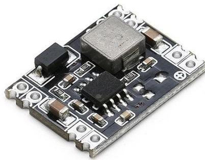
Figure 1.4: 5V to 3.3V Step Down Voltage Regulator
