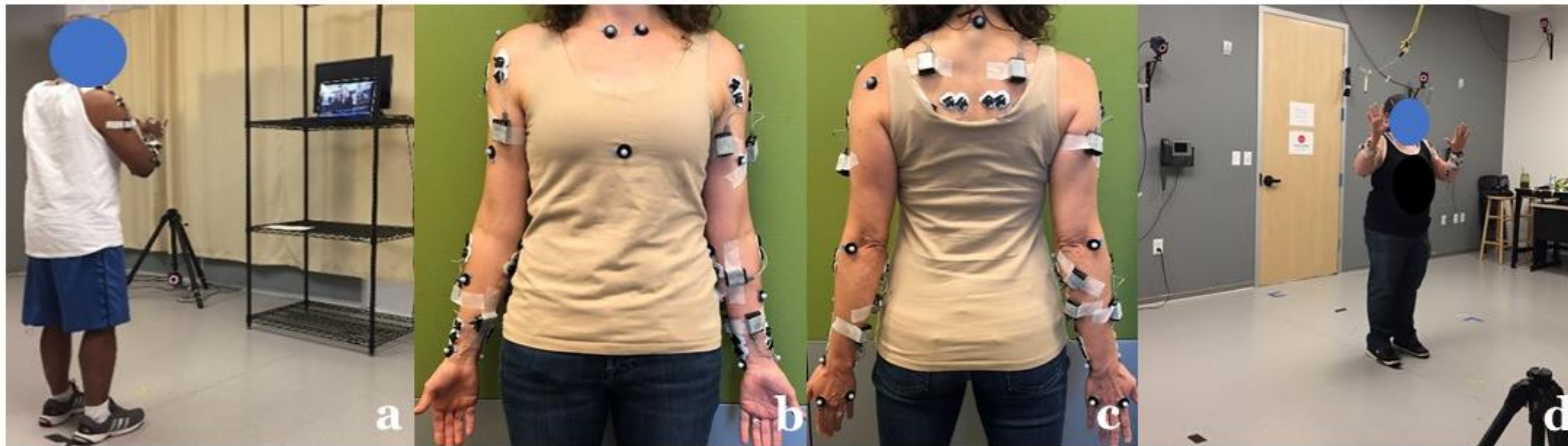
Figure 2.2. a) Participants signed from a video source in sign language with audio and closed captioning. b) Anterior and c) posterior views of electrode placement for surface EMG and surface marker placement for motion capture. d) A motion capture system tracking surface markers on upper limb segments.
