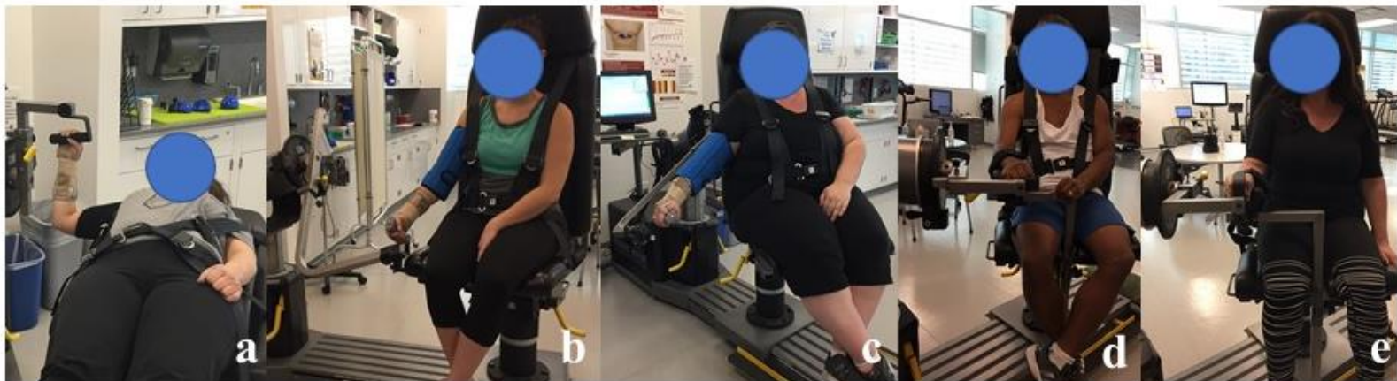
Figure 2.1. Isometric a) shoulder internal-external rotation, b) shoulder flexion-extension, c) shoulder abduction-adduction, d) wrist flexion-extension, and e) wrist radial-ulnar deviation strength assessment using an isokinetic dynamometer.
