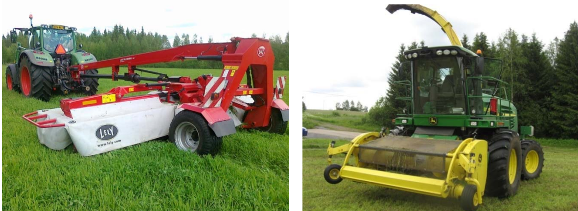
Figure 3.1. Lely Splendimo 550 P disc mowing machine and John Deere 7250i harvester were used in the topping farm trial in Eastern Finland (Photo by P. Kurki).
