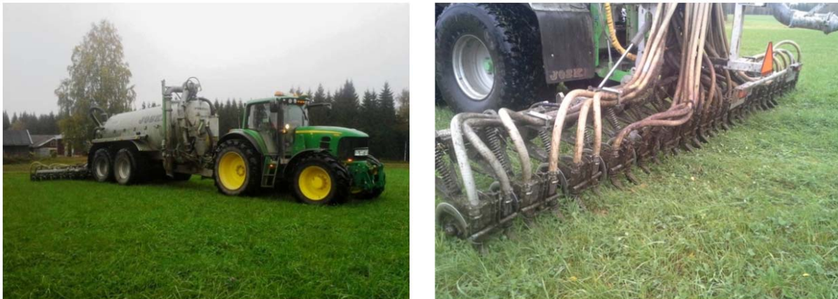
Figure 3.2. The slurry was injected directly into the sward by Joskin slurry tanker in the manure farm trial in Eastern Finland. (Photo by A. Laamanen).
