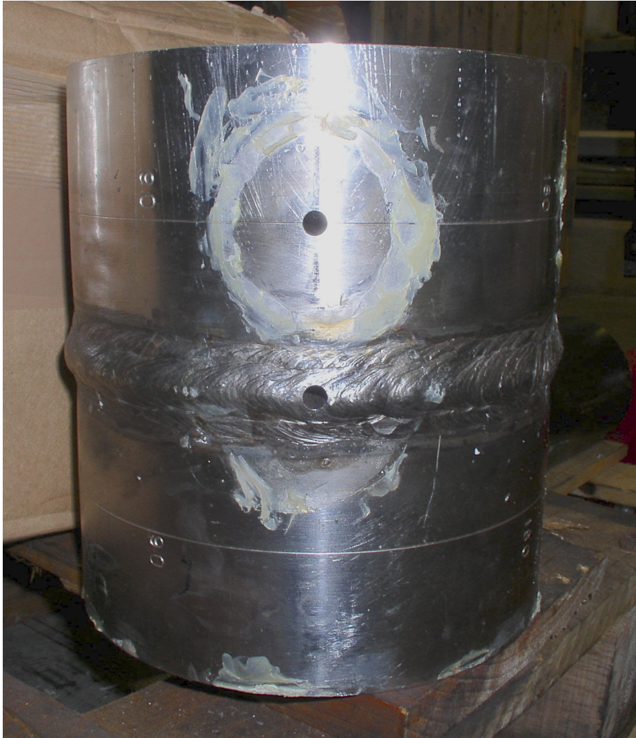
Figure 2: Showing completed short pipe mock-up after iDHD measurements in the as-welded state
