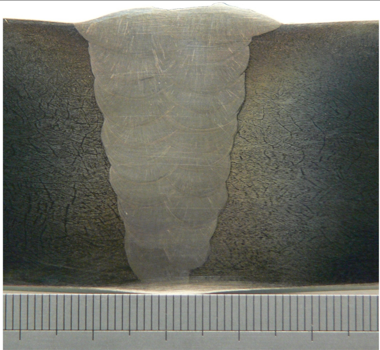
Transverse micrograph from two-capping pass pipe CY7/CY6
