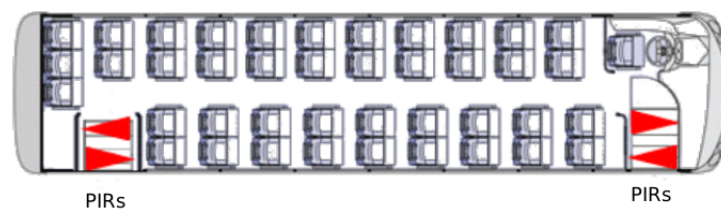
Figure 3. Sensor application in a bus. PIRs, passive infrared sensors.
