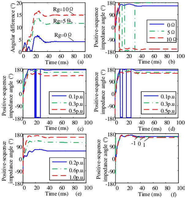
Fig. 10. Angular features of  $\Delta Z_{1\phi}$  with different influence factors. (a) Angular differences of positive-sequence voltage, (b) Fault resistances, (c) Active power reference values, (d) Reactive power reference values, (e) Load currents, (f) Control strategies.
