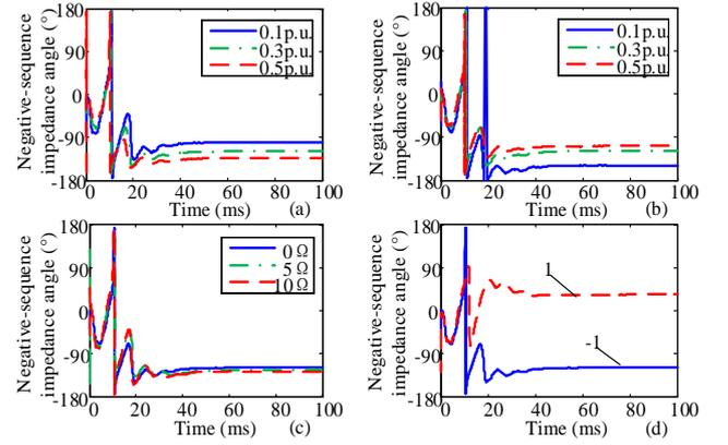
Fig. 11. Angular features of  $\Delta Z_{2\phi}$  with different influence factors. (a) Active reference values, (b) Reactive reference values, (c) Fault resistances, (d) Control strategies.
