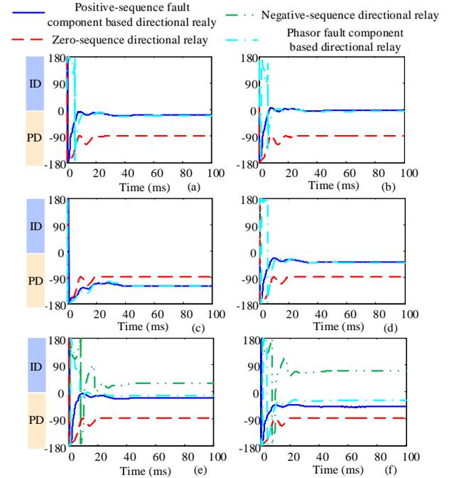
Fig. 12. Performance of different types of fault component based directional relays under different influence factors. (a)  $K=0$ ,  $R_g=5\Omega$ , (b)  $K=0$ ,  $R_g=10\Omega$ , (c)  $K=0$ ,  $k_3=0.2$  p.u., (d)  $K=0$ ,  $k_3=1.0$  p.u., (e)  $K=-1$ ,  $Q_a^*=0.1$  p.u., (f)  $K=-1$ ,  $Q_a^*=0.5$  p.u.
