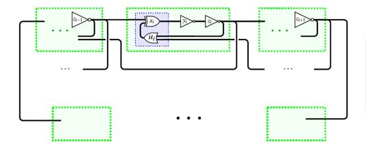
**FIG. 1.** The basic unit (within the green rectangle) receives input from the second inverter of both the previous and next units. Besides two inverters, each unit comprises a logical gate (blue rectangle) coding for the Boolean function  $f(z_{i-1}, z_i, z_{i+1})$ , see (1). The overall structure is periodic:  $i \in \{1, ..., n\}$  and i is considered modulo n.
