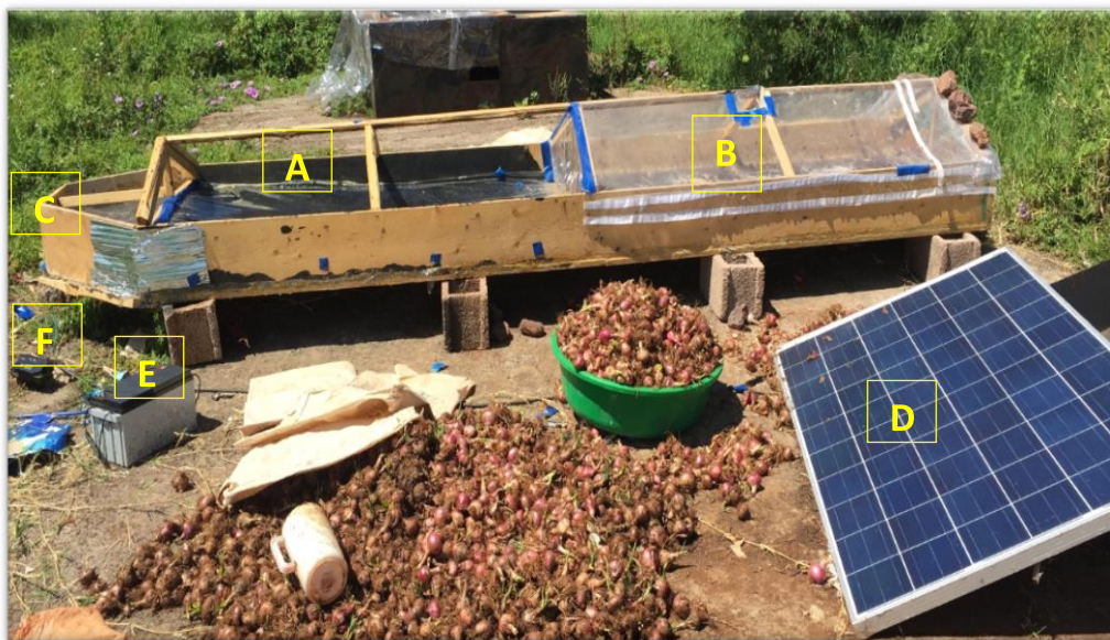
Figure 1. A solar tunnel dryer setup constructed for onion curing: (A) solar collector; (B) drying chamber; (C) axial fan; (D) solar panel; (E) solar battery and (F) solar charge controller.
