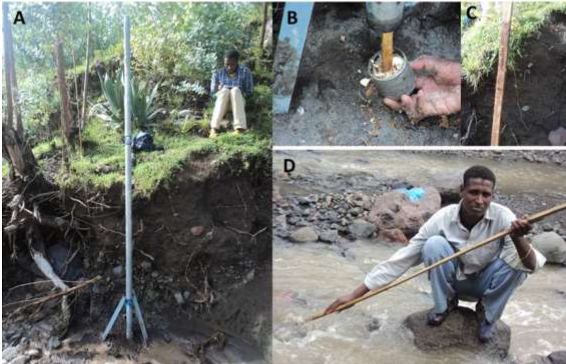
Fig. 3: Crest stage gauge (A), sawdust being placed in the bowl of the lower cap before and after measuring peak stage (B), remnants of sawdust on wood staff indicating the highest peak stage of the flood (C), and wood staff being cleaned for the next flood (D).
