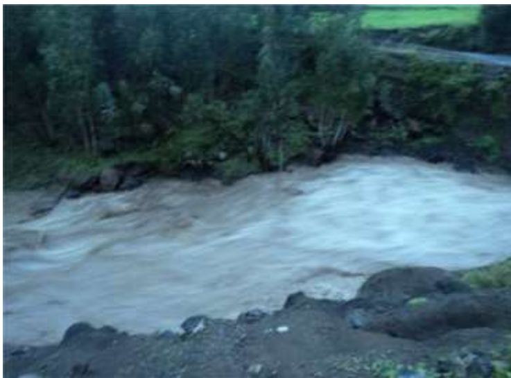
Fig.4. Daily rainfall of 21.1 mm in Wera catchment (23/8/2013) resulted in a flash flood peak of 128 m 3 per second. Crest stage gauge appears in the middle of the opposite bank.
