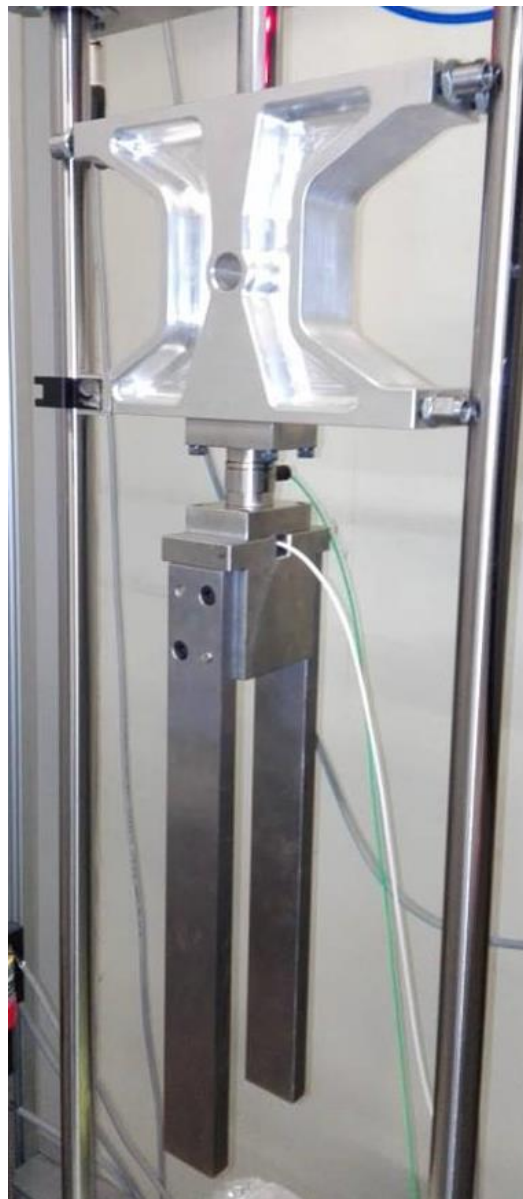
Figure 3.20 - Final arrangement of the anvil-impactor assembly.
