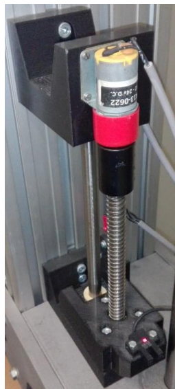
Figure 4.10 - Velocity acquisition sub-system.
