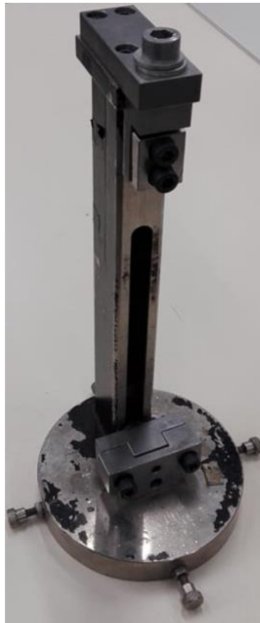
Figure 5.4 - Rosand machine's specimen fixing structure.
