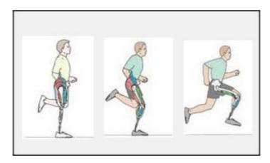
Figure 7. Amputee Running. From left to right: 'stance' phase, 'absorption' phase and 'swing' phases (Gailey 2002).
