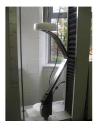
Figure 33. Prosthetic Blade Loading
