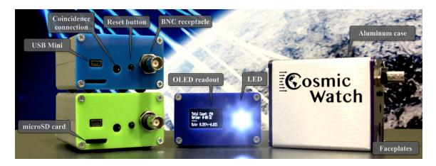
Figure 1. An array of the Desktop Muon Detectors.
