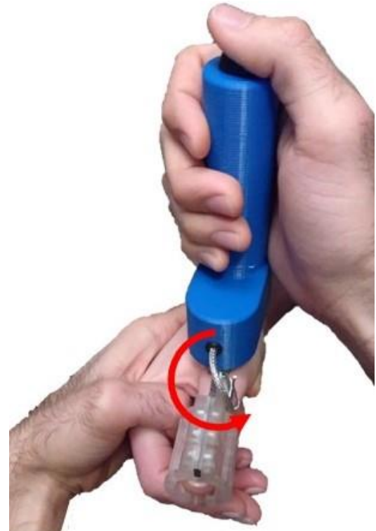
Figure 2: Final built prototype of the thumb UCL testing device being used to test a thumb. When the motor turns, the thumb is moved in the direction of the arrow, thereby generating a torque on the MCP joint.
