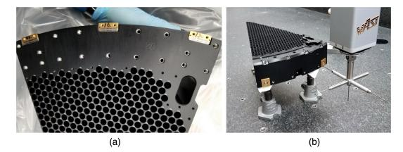
**Fig. 5** (a) Three slots are available for petal-ring mount pad installation on a petal. By loosening the pad, the gauge blocks it houses can be slid out and hot swapped. Each pad is hand-measured and numbered to match the depth of each slot. (b) The three-slot scheme was found to be an over-design. Only the left and right slots were used, the middle left empty for aligning all petals. The petal-ring mount pad and GFA-FPP mount plate were surveyed on a CMM before petal alignment in the FPR.
