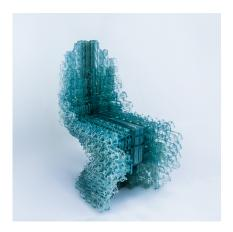
The prototype was fabricated at Nagami, a small company in Avila, Spain, a company specialized in large scale 3D printing. Transparent PLA pellets mixed with cyan coloring (Figure 11) was used as the extrusion material. The equipment at Nagami consists of an ABB IRB4600 industrial robot with a mounted customized plastic pellet extruder. It uses a stepper motor with an independent controller (not driven by the robot controller) (Figure 12).
