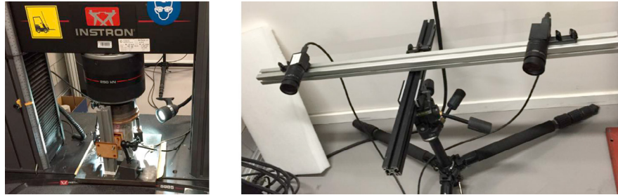
Figure 4. The DIC setup and Instron machine.
