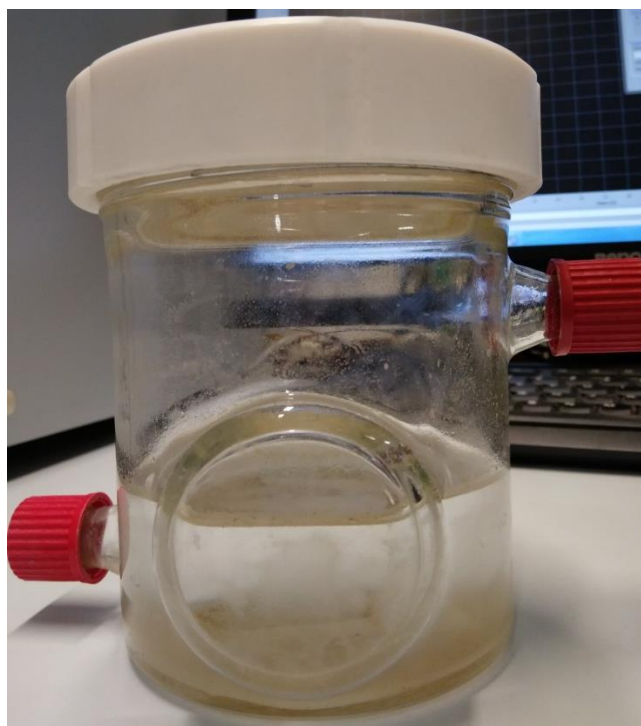
Figure 23. Borosilicate reactor for water redox batch reactions. Light is irradiated on the side window and two side outlets are used for purging and taking the gas products.
