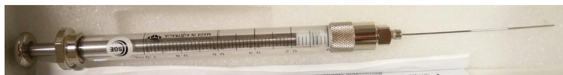
Figure 19. Photograph of the gastight syringe used during photocatalysis experiments.
