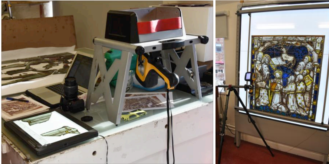
Figure 6.2 Analyses by handheld pXRF were carried out using a test stand (left) whenever possible; if the glass pieces were not removed from their lead cames, the analyses were carried out using a tripod (right) or handheld.
