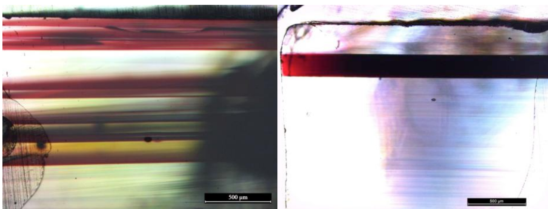
Figure 8.28 Two non-original red glass pieces with low lime composition. Most of the red glasses in this group have Type A structure, like the glass piece on the left (10e-R2). One non-original red has Type B structure (on the right, 3b-R5).
