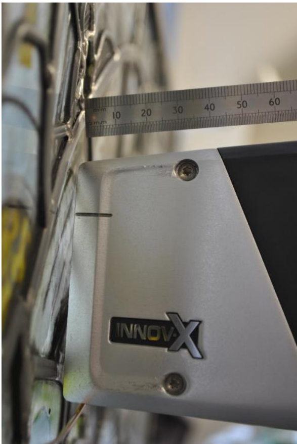
Figure 5.6 Lead comes can protrude multiple millimeters, and together with the use of small pieces of glass, prohibit the placement of the pXRF spectrometer directly on the surface of the glass for analysis. The glass in this image has been recently conserved and re-leaded, and the modern lead comes in these panels protrude by about 2-4mm.
