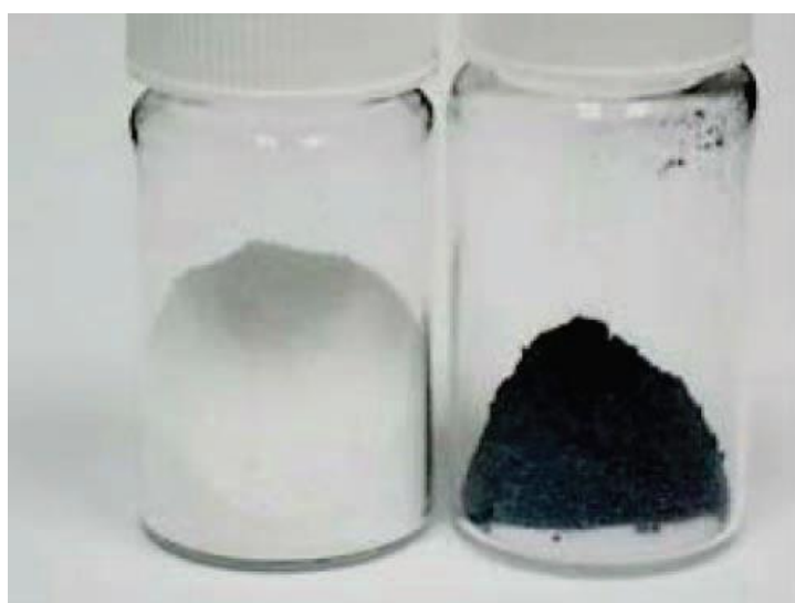
Figure 1.4. The colour of TiO 2 before and after hydrogenation at 200 °C for 5 days. Reproduced from [62].
