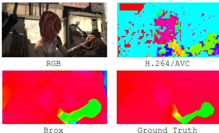
Figure 3.1: RGB frame from the MPI-Sintel dataset and pseudocolored images of the motion information amplitude. The H.264/AVC MB motion vectors are correlated with Brox optical flow extracted from decoded video frames [123][124] and the ground-truth motion available for this synthetic video.
