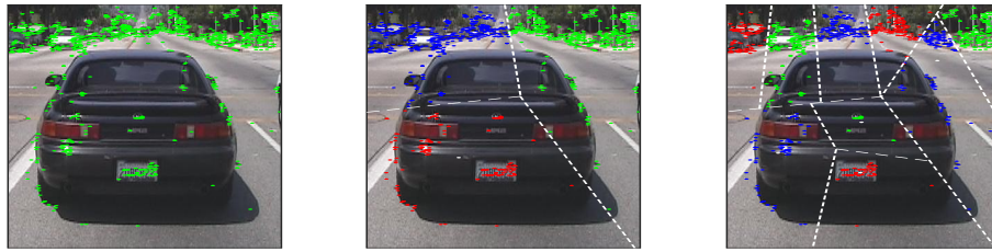
Figure 2.1: Three-level Voronoi partitioning for an image from Caltech Cars dataset. For illustration purposes, SIFT descriptors are color-differentiated for each cell.
