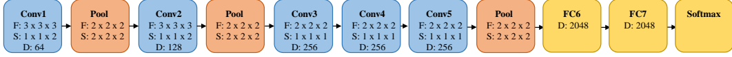
Figure 3.5: 3D CNN architecture: the blue, orange and yellow blocks represent convolutional, pooling and fully-connected layers; F is the filter size for the convolutional layers (or window size for pooling), formatted as width \times height \times time; S is the filter/window stride; D is the number of filters (or number of hidden units) for the convolutional and fully-connected layers.
