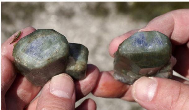
Figure 1. Naturally occurring cordierite specimens found in the Norwegian coastal area. The specimens have the characteristic blue colour. Thin platelets of specimens like this of high optical quality could have been used by Vikings as polarization filters to determine the sun position during overcast days[2]. Photograph ©Jan Kihle
