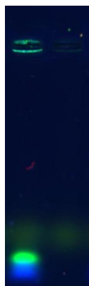
Figure 4-20 Analysis of the incorporation of fluorescently tagged DNA-enzyme conjugates to the DNA nanoball. Analysed by 1% 1 X TBE agarose gel electrophoresis.
