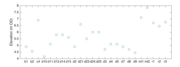
Figure 4.7 Pond bed elevation (metres) in relation to mean sea level (OD – ordnance datum)
