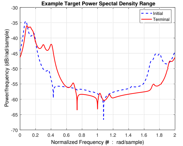
Fig. 3: Target Fourier response based on extended target assumption, modelled by AR process.
