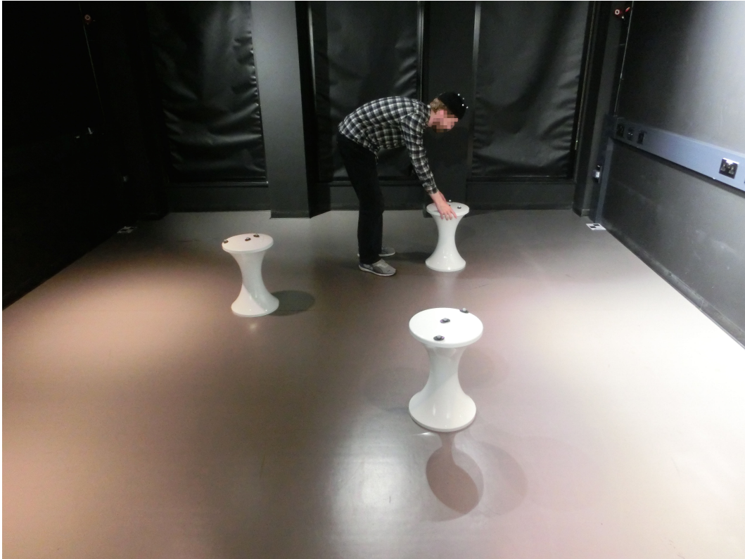
Figure 5.2: Participant placing the three objects in the recall stage. Plastic stools were used as objects for the study. Three retroreflective markers were attached to each stool for optical tracking.
