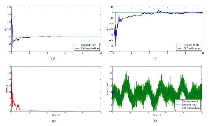
Fig. 8. Representative result for the simulation of the placenta surface estimation. In (a) and (b) the estimation of the altitude  $\theta$  and the azimuth  $\gamma$  of the placenta normal  $\mathbf{n}$  is visualized, respectively. The angular error in the estimation of  $\mathbf{n}$  with respect to the ground truth  $\mathbf{n}_{th}$  is shown in (c). This error equals  $\arccos(\mathbf{n} \cdot \mathbf{n}_{th})$ . The estimated distance is depicted in (d).
