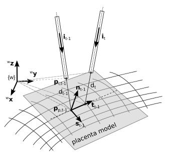
**Fig. 5.** Approximation of the placenta surface by a plane with normal  $\mathbf{n}$ . The distance sensor measures the distance d from the instrument tip  $\mathbf{p}_i$  along the instrument direction  $\mathbf{i}$  until the intersection with the placenta at point  $\mathbf{p}_p$ .
