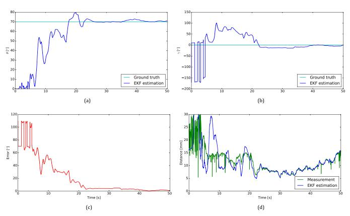
Fig. 12. Representative result of placenta surface estimation algorithm; (a), (b) respectively estimation of altitude  $\theta$  and azimuth  $\gamma$  of the placenta normal  $\mathbf{n}$ ; (c) angular estimation error of  $\mathbf{n}$  with respect to the ground truth; (d) filtered distance measurement, together with the raw distance measurement (including outliers).
