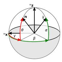
**Fig. 6.** Parametrization of **i** with altitude angle  $\alpha$  and azimuth angle  $\beta$  (green) and parametrization of **n** with altitude angle  $\theta$  and azimuth angle  $\gamma$  (red).
