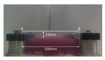
**Fig. 14.** Definition of the line-tracing task. The operator is asked to move the instrument from point A to point B while maintaining a constant distance of 10 mm to the placenta surface.
