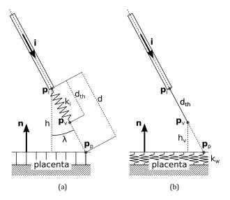
**Fig. 9.** Different haptic guidance approaches. In (a) a virtual spring is implemented between point  $\mathbf{p}_i$  and point  $\mathbf{p}_{\nu}$ . This spring will compress when  $\mathbf{p}_{\nu}$  touches the rigid placenta surface. In (b) the virtual point  $\mathbf{p}_{\nu}$ , which is rigidly connected to the instrument, compresses the elastic placenta surface.
