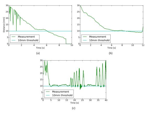
**Fig. 13.** Instrument-placenta distance as a function of time. (a) and (b) show the distance when the operator moves carelessly towards the surface, respectively without and with assistance from the haptic guidance. In (c) the operator moves around near the placenta surface in a relatively rough fashion, while the guidance ensures sufficient clearance between the instrument tip and the placenta.
