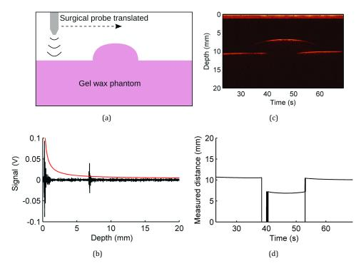
**Fig. 4.** (a) Schematic of a scan over a vessel phantom. (b) Single ultrasound A-line, corresponding to 45 s in (c), showing the distance threshold (solid red). The reflected signal is visible at around 6 s. (c) M-mode ultrasound image of the scan vessel. (d) Measured distance to the phantom surface.
