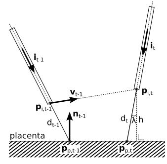
**Fig. 7.** Representation of the distance prediction, showing the instrument pose and the associated distance measurement at two consecutive time instants. The representation is a projection onto a plane parallel to  $\mathbf{n}_{t-1}$  and  $\mathbf{i}_t$ .
