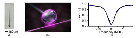
Fig. 1. (a) A microscope image of a typical microsphere-cantilever. (b) Artist's impression of the microsphere-cantilever, which is brought close to, but never touches, the tapered optical fiber underneath it. The evanescent fields of the WGM and tapered fiber are illustrated. (c) Monitoring the transmission *t* through the taper as the laser frequency is scanned reveals a WGM resonance (black), fitted with a Lorentzian function (blue) with a FWHM of 6.8 MHz.
