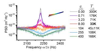
Fig. 7. PZT cooling of a microsphere-cantilever with a lower  $Q_m = 280$  than in Fig. 6 and higher noise floor, showing squashing with large feedback gain,  $g_c$ . The mechanical mode is shown as an inset. Data was taken at atmospheric pressure, with curves fitted using Eq. 2 & Eq. 3 to infer the mode temperatures, with less than 10% uncertainty unless stated.
