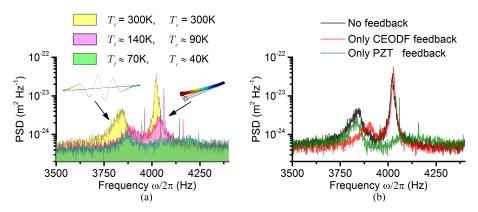
Fig. 8. (a) Simultaneous cooling of a taper mode at  $T_t$  and the microsphere-cantilever mode at  $T_c$  using both the PZT and the CEODF, performed at atmospheric pressure. Mode temperatures are approximated by integrating the area under the respective peaks. (b) Cooling with *only* the CEODF or the PZT scheme, each optimized for the taper mode and cantilever mode respectively, can influence the transduced PSD of the other oscillator.
