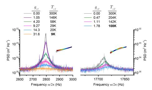
Fig. 6. PZT feedback cooling of the fundamental mode of the microsphere-cantilever with  $Q_{m1} = 370$ , reaching  $T_{c1}$  at varying feedback gains  $g_{c1}$ . The second mechanical eigenfrequency at 17.73 kHz, with  $Q_{m2} = 640$ , is simultaneously cooled to  $T_{c2} = 108$  K. Mechanical mode shapes are shown as inset diagrams. Data was taken at atmospheric pressure, with curves fitted using Eq. 2 to infer the mode temperatures  $T_{c1,c2}$ , with uncertainties of less than 10%.
