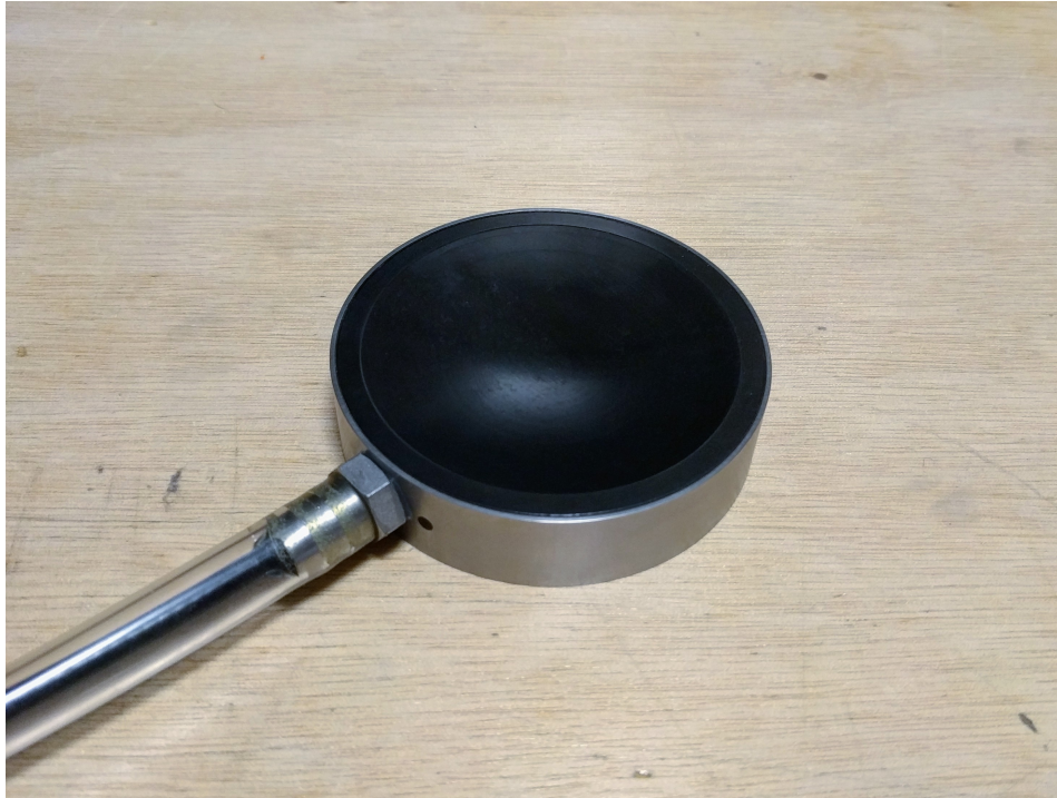
Figure 1.1: Sonic Concepts H151 spherically focussed ultrasound transducer.
