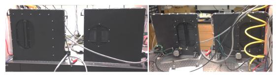
Figure 17: The shutter assemblies shown in the closed position with the exposure shutter on the left and the NIR shutter on the right. The views show the front (left) and reverse (right) sides of the shutters. The fiber illuminator LED is visible in the exposure shutter door front view. The motor and inflatable seal mechanism is visible in the reverse view.
