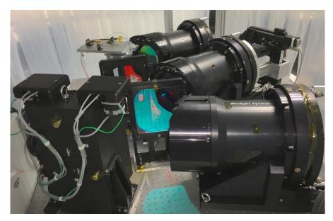
Figure 24: The DESI spectrograph in integrated alignment using a tooling slit source. The cryostats are not attached to the cameras and their focal planes can be measured with a microscope. The dichroic filters are visible (blue and red) and the furthest, NIR channel camera VPH is visible (green). The nearest camera is the red channel. The shutters and baffles are integrated at a later time.
