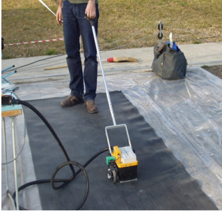
Fig. 2. Employed GPR equipment.
